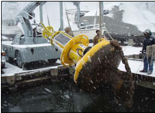
The NOAA Chesapeake Bay Office pulls the Patapsco buoy out of the water each winter to prevent ice damage to the buoy's water quality sensors. Credit: NOAA.
